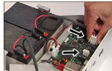
**2** Detach the battery cables from the controller board.
